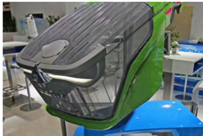
Distinctive special tractor radiator grille for the Fendt 200 V/F/P Vario, supplied ready-to-fit by SCHÄFER Perforated Metal
