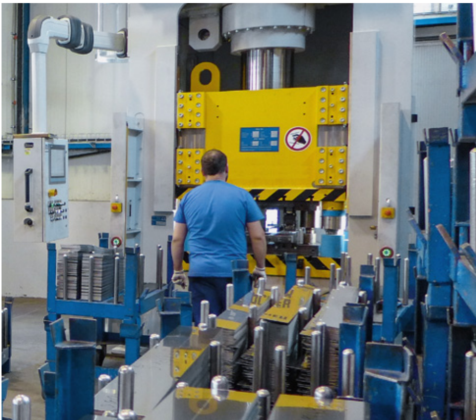
Deep drawing press for forming operations.
